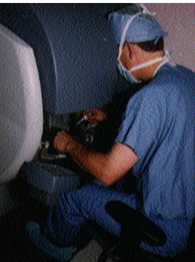
Christopher Kane operating laparoscopically from the console of da Vinci™ Surgical System. His movements are translated with imperceptible delay to the robotic system, which executes the surgical procedure.
